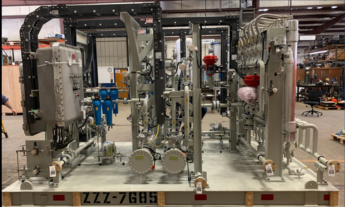
Air compression system with nitrogen filtration
